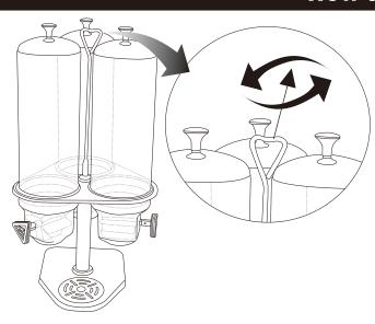
The speed of the rotation can be adjusted by turning the revolving rod clockwise (to be tight) or anticlockwise (to be loose).
